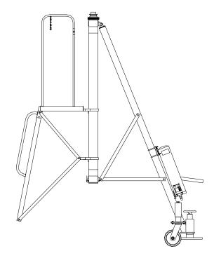
Our Fixed Height Tripod Jacks are used on and for specific aircraft jacking applications during normal aircraft maintenance checks. Our tripod jacks are designed and built to withstand harsh environmental conditions, rugged use and to provide many years of continuous service.
