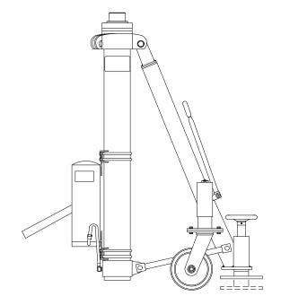
Our Fixed Height Tripod Jacks are used on and for specific aircraft jacking applications during normal aircraft maintenance checks. Our tripod jacks are designed and built to withstand harsh environmental conditions, rugged use and to provide many years of continuous service.
