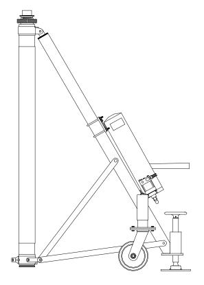
Our Fixed Height Tripod Jacks are used on and for specific aircraft jacking applications during normal aircraft maintenance checks. Our tripod jacks are designed and built to withstand harsh environmental conditions, rugged use and to provide many years of continuous service.
